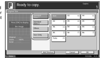
If [Size Entry] is selected, press [+] or [-] to specify the horizontal size (X) and the vertical size (Y). Press [# Keys] to enter the size directly using the numeric keys.
