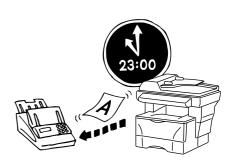
**NOTE:** Timer-based Transmission is not available in Direct Transmission mode. The fax memory can hold up to 30 jobs for timer-based transmission at once.
