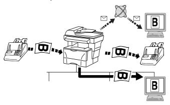
**NOTE:** If fax forwarding fails, the received documents are printed from the FAX System and deleted from memory.
