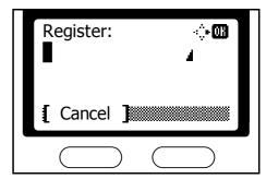
**NOTE:** Encryption keys consist of a series of any 16 characters consisting of numbers (0 to 9) and the letters A through F.
