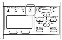
Press **Stop/Clear** to clear the Error indicator if it remains lit even after you take corrective action and resolve the error.
