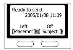
2 Choose the fax mode. Select from memory transmission mode or direct transmission mode. (The default setting is memory transmission mode.) To choose direct transmission mode, follow the procedure given in *Direct Transmission* on page **4-7**.
