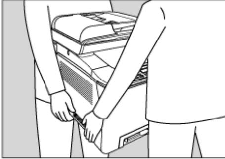
**3** Remove the protective materials attached on the machine's exterior. Do not remove tapes going into the inside of the machine.
